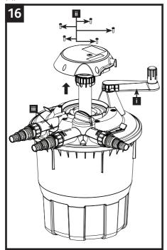
7.1.5 Grip the electrical housing and gently pull up to remove the electrical housing. Turn the housing upside down and place on a dry level surface.
