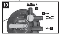
Place the pump in the pond in a suitable location and position the end of the outlet hose so that filtered water returns to the pond.
