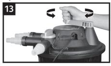
6.4 Turn the diverter valve to the waste position (Fig. 14). You will hear a "click".
